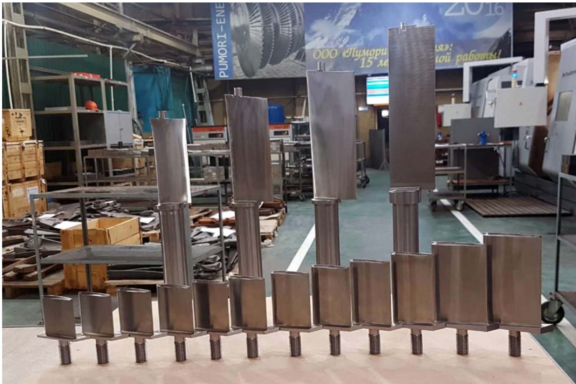
Vanes of stages 0-11 and inlet guide vanes Gas turbine GTN-16 (UTZ design)
